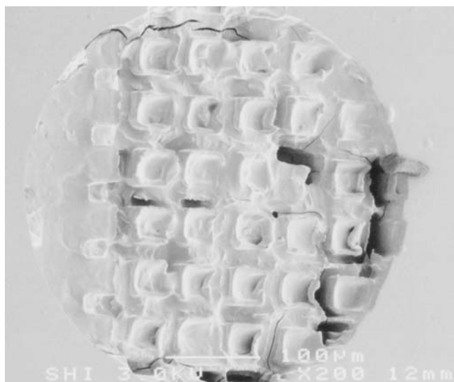
Fig. 14 Serious thermal damage to the PMMA resist by unreasonably increasing the dose to 52.6 A min, consistent with the saturating phenomenon observed in Fig. 13. The development could not be carried out to create microstructures
