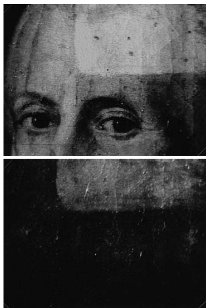
Fig. 7 Image ( top ) and UV reflectography ( bottom ) of a laser-cleaned area on an 18th century oil painting. In the reflectance spectrum, the dark area represents the initial varnish in which the various photodegradation products absorb strongly the incident light (365 nm), whereas the laser-uncovered, "fresh" varnish is clearly characterized by higher UV reflectivity
