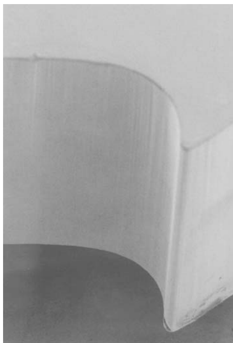
Fig. 3 SEM picture of the high aspect ratio structure made of PMMA by the LIGA process. Typically, the structural height (depth) is 100–500 \mu\text{m} and the feature size is 2–20 \mu\text{m} ; thus, the aspect ratio is between 5 and 100
